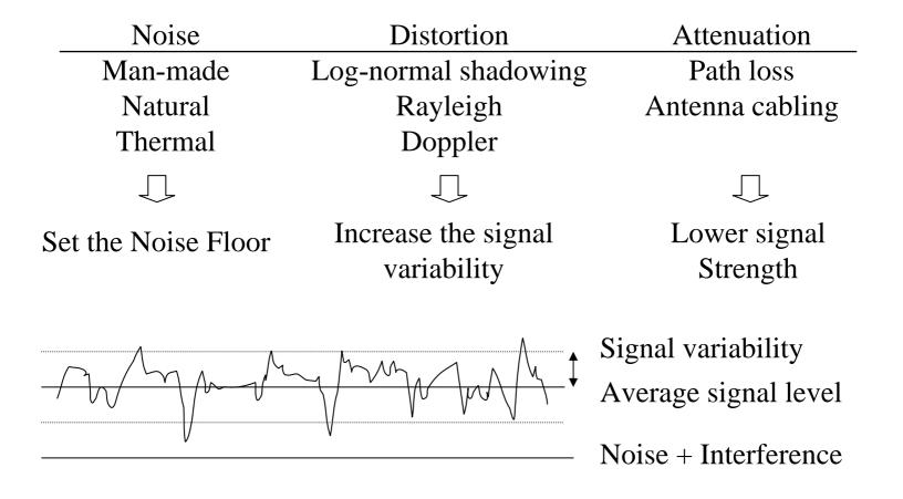
Average signal level - Signal variability > Noise + Interference
